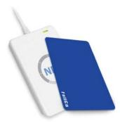
The ACR122U NFC Reader is a PC-linked Contactless Smart Card Reader/Writer developed on the 13.56MHz Contactless Technology. It is the world's first CCID Compliant Contactless Card Reader/Writer that follows both ISO14443 and ISO18092. It is designed to support not only MiFare and ISO14443 Type A and B Cards but also FeliCa and NFC tags.
